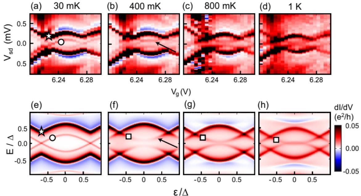
Temperature dependence of Andreev spectra in a superconducting carbon nanotube quantum dot
