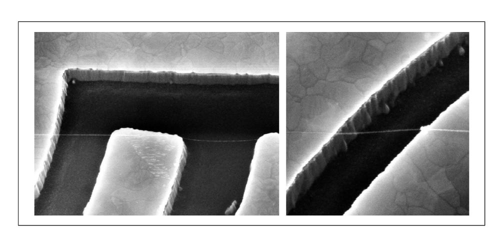
successful nanotube growth across superconductor layers and trenches • metal  $T_{\rm c} \simeq 800 \, {\rm mK}$  after CVD process fabrication and testing ongoing
