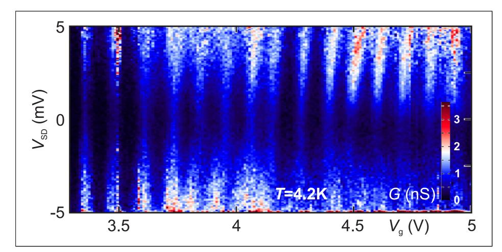
• first suspended CNT quantum dots with Pt contacts (i.e. normal metal; tests at  $T = 4.2 \,\mathrm{K}$ )
