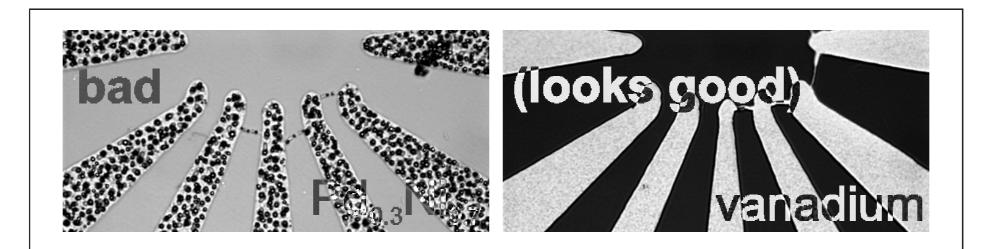
• CVD: 10min, 900°C, CH<sub>4</sub> and H<sub>2</sub>: for a metal thin film "as bad as it gets"
